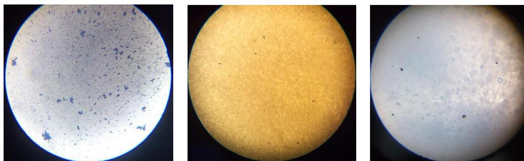
314 (a) NS liquid (b) NS liquid with surfactant (c) NS liquid with UV
