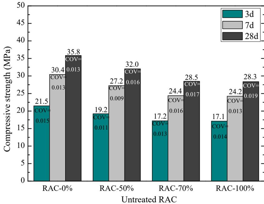
Fig. 12 Compressive strength of untreated RAC
