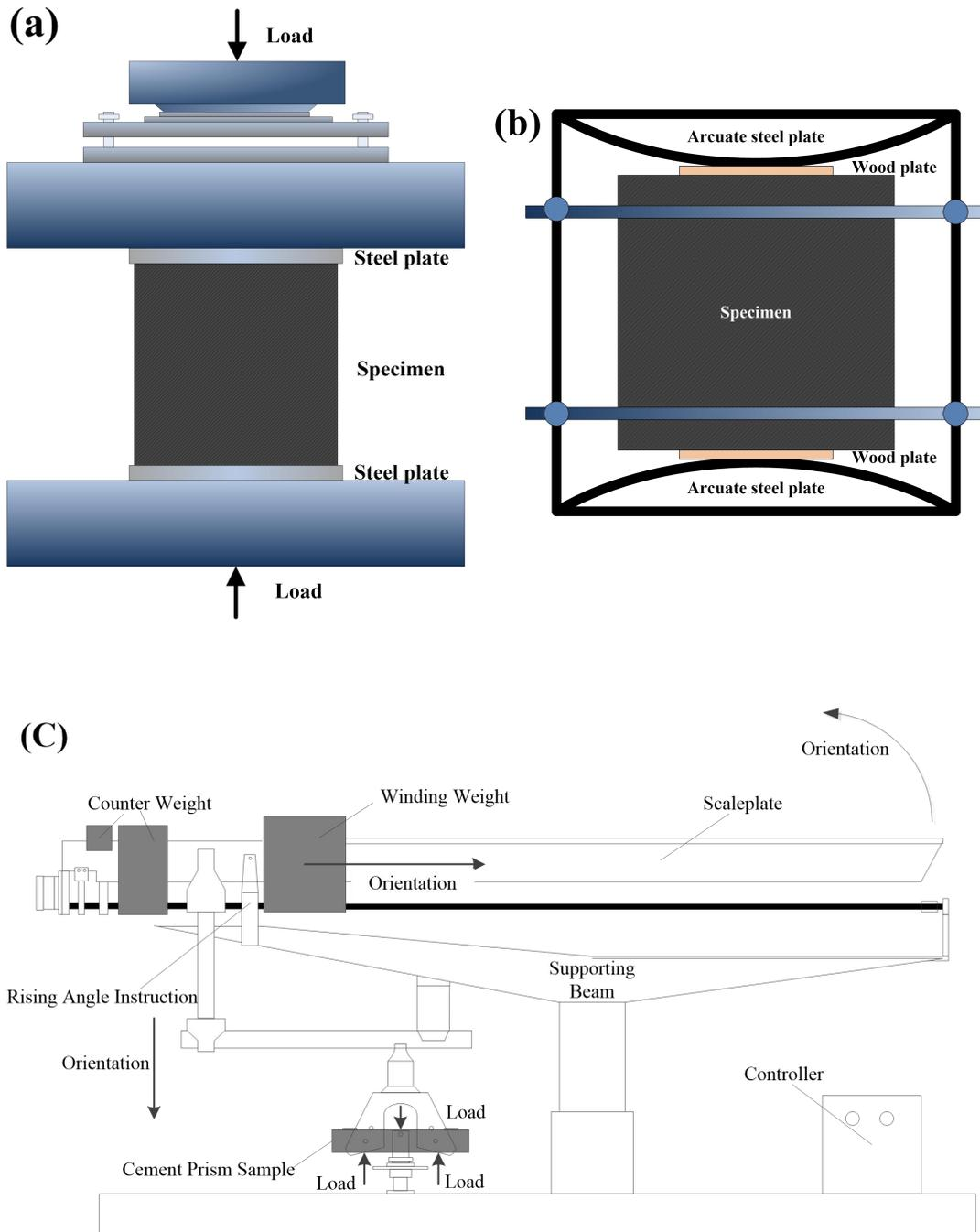
Fig. 4 Test setups: (a) compressive testing, (b) split tensile test, (3) schematic view of standard cement mortar flexural tensile test
