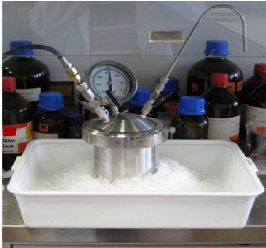
Figure 5.2.1.2 Nitrogen cavitation device for isolating cell membranes. Nitrogen gas is delivered under pressure (1000-1500 psi) into the cavity to “bomb” the cells into membrane fragments. The cavitation device containing the fragmented cells is left on ice for 15 minutes
