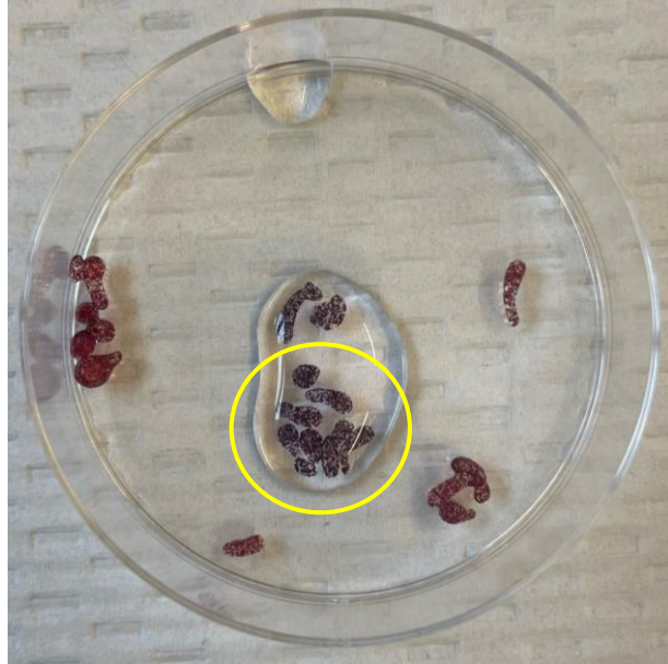
Figure 0.8 Extruded microbeads with high concentration of Alginate (4% w/v) in presence of the ionic exchange resin. In the centre, the microparticles took on a blue/purple colour because they were wetted by a basic solution. Yellow circle indicates the beads treated at different pHs and showing different intensity of red.
