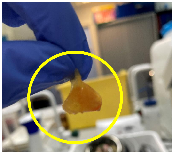
Figure 0.24 In the yellow circle the clog made after the centrifugation because of the droplets instability.
