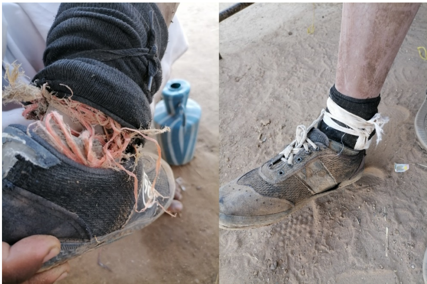
Figure 1: Ahmed's broken prosthetic leg fixed with a traditional rope.
