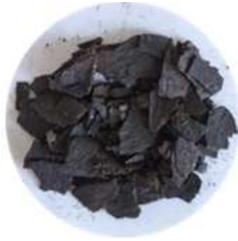
Figure 1. Prepared HA-F based PCM microcapsules
