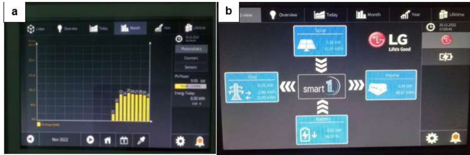
Fig. 2 Control unit readings, a) Daily electricity consumption where the average was 90 kWh b) Distribution of electricity gain and consumption for one day.
