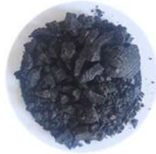
Figure 1. Prepared nonadecane@HA microcapsules
