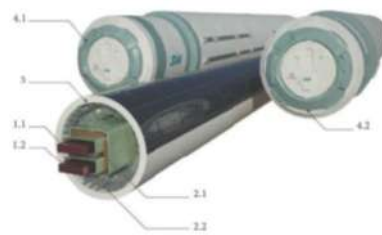
Fig.1 – GPV design: 1.1 and 1.2 – belt flywheels; 2.1 and 2.2 – magnetic suspension systems and linear electric motor; 3 – body; 4.1 and 4.2 – containers with cargo (visualisation)
