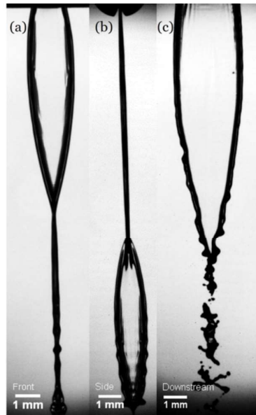
Figure 3. Rim formation mechanism: (a) front view - primary Sheet, (b) side view - secondary sheet, and (c) breakup in the downstream region.
