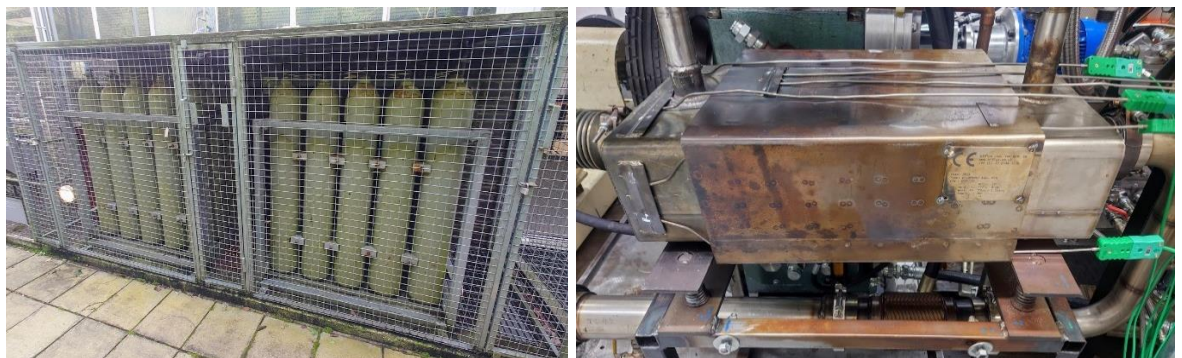
Figure 5.5 Photographs of the two sets of 15 bottle high pressure cylinder banks (left) and the Hiflux recuperator (right) utilised on the SCCRE test bed.
