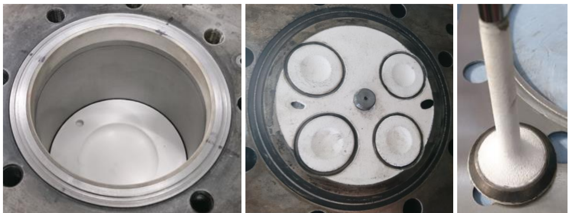
Figure 5.3 Photographs of the ceramic coating utilised on the surfaces of the piston crown (left), upper liner cuff (left), cylinder head flame plate (middle), valve face (middle), and valve stem (right).
