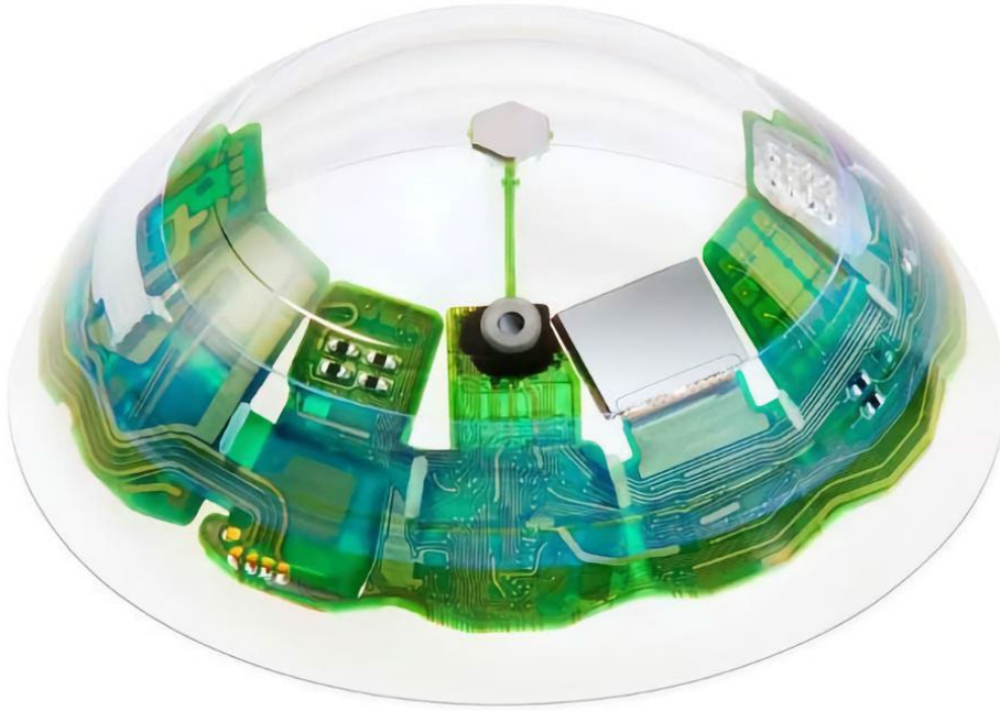
Figure 1: The prototype Mojo Vision smart contact lens with a 14,000 pixels per inch MicroLED display, the world's smallest at just 0.5 mm in diameter, and densest with a pixel-pitch of just 1.8 microns, 5GH ultra-low latency radio to stream AR content, continuous eye tracking via custom-configured accelerometers, gyroscopes, and magnetometers, medical-grade in-lens batteries, and eye-controlled user interface (2).
