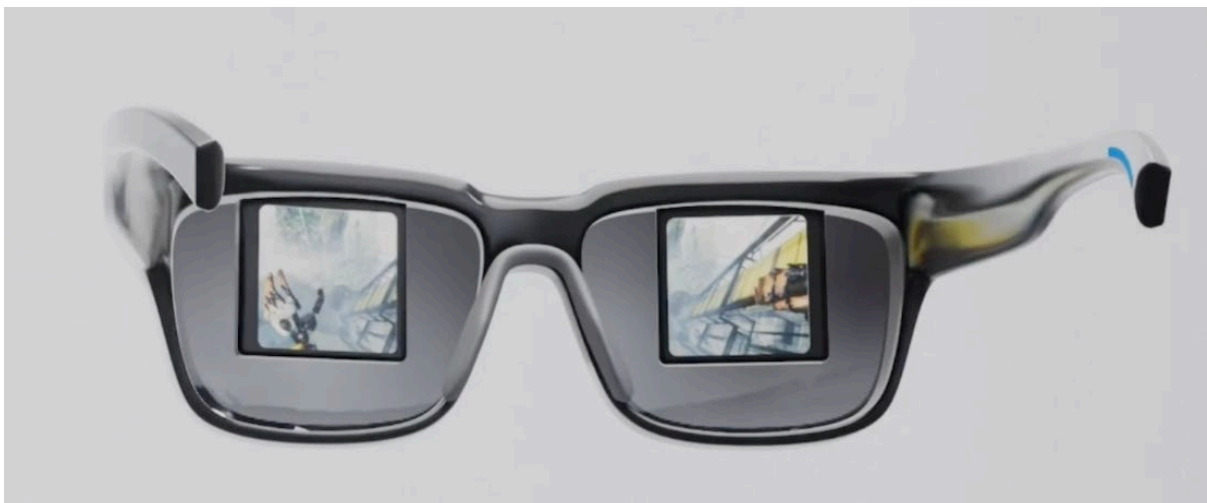
Figure 2: The vision enhancement technology by Innovega is made of display glasses and a smart lens that picks up the images and media from the eyewear display and projects it directly on the retina.
