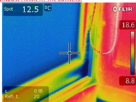
THERMOGRAM 5: ONE SASH WINDOW IN THE LIVING ROOM, SHOWING THE AIR LEAKAGE TAKING PLACE THROUGH THE WINDOW FRAME AT THE CORNERS.
