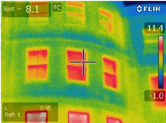
THERMOGRAM 1: THE FRONT WALL FROM THE OUTSIDE, SHOWING THE HEAT LOSS TAKING PLACE THROUGH THE SINGLE GLAZED SASH WINDOWS.
