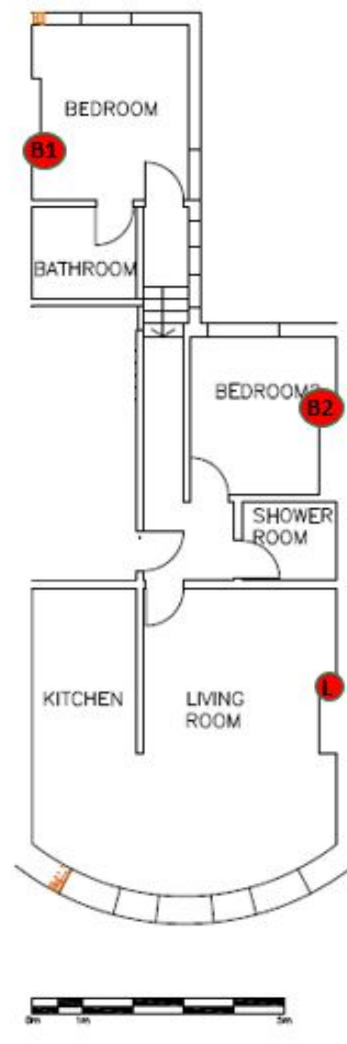
FIGURE 0.9 FLOOR PLAN OF THE CASE STUDY DWELLING N.2 (1 ST FLOOR) WITH ANNOTATED POSITION OF TEMPERATURE AND RH DATA LOGGERS IN THE LIVING AREA (L) AND BEDROOM AREA (B1: MAIN BEDROOM; B2: GUEST BEDROOM)
