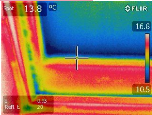
11-6 THERMOGRAM 6: ONE SASH WINDOW IN THE LIVING ROOM, SHOWING THE AIR LEAKAGE TAKING PLACE THROUGH THE WINDOW FRAME AT THE CORNERS.
