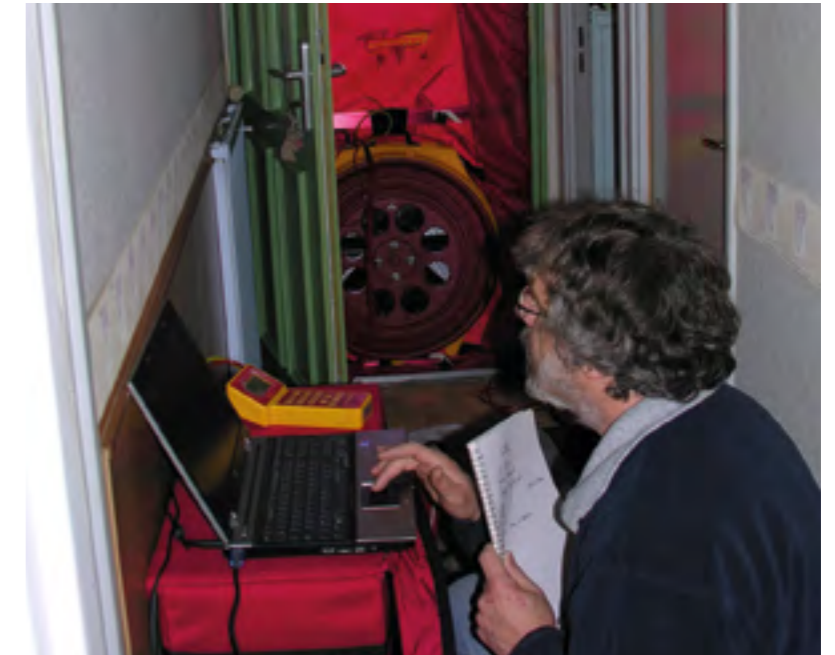
A Blower-door test in Outreau (January 2013).
