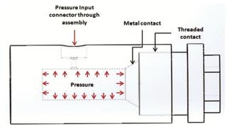
Fig. 1 — CAD model of pressure chamber
