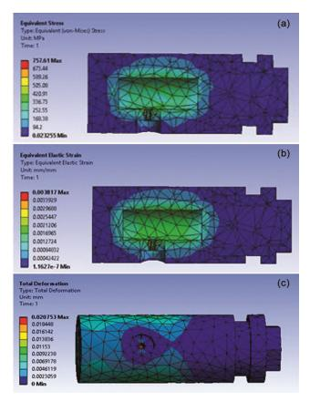
Fig. 4 — (a) Maximum equivalent stress (b) Maximum equivalent strain and (c) Total deformation in pressure chamber
