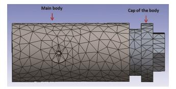
Fig. 2 — Meshing of pressure chamber
