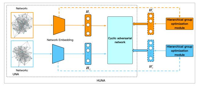
Fig. 2. Diagram of the overall framework.  $H_1$  and  $H_2$  denote low-dimensional vector representations of nodes learned by network embedding methods in  $Network_1$  and  $Network_2$ , respectively.  $H_1^i$  and  $H_2^i$  denote the low-dimensional vector representation of the group obtained by the nodes in  $Network_1$  and  $Network_2$  through our proposed hierarchical group optimization module, respectively.
