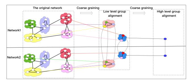
Fig. 7. Flow diagram of the hierarchical group optimization module. The black bold line represents the link edge between nodes or groups, the colored thin lines represent the coarse-grained process or group gathering process, the different node colors represent the different groups divided, and the black dotted line represents the entity alignment process.
