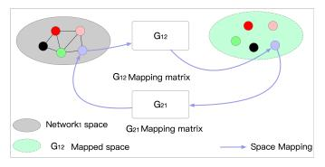
Fig. 6. The diagram of node reconstruction. After nodes in network 1 are mapped by  $G_{12}$ , they can be reverted to network 1 by  $G_{21}$  ideally. After continuous training to reduce the reconstruction loss.
