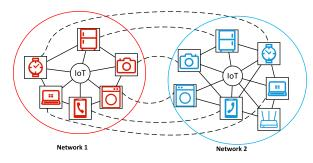
Fig. 1. Diagram of network entity alignment in IoT. Each network can be abstracted into a graph. Nodes represent IoT devices, and edges represent connections between devices. Different colors represent different networks, and devices connected by dotted lines are similar device pairs in different networks identified by network alignment.
