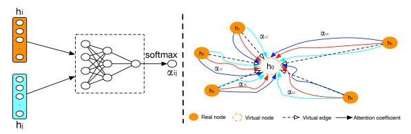
Fig. 8. The left image is the schematic diagram of the Graph Attention network structure. The right image is a diagram of information aggregation. The entity node is the real node divided into the unified group, the virtual node represents the group after the aggregation, and the dotted line represents the virtual connection edge from the real node to the virtual node.
