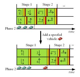
Fig. 9: Attack strategy of the 'last vehicle'. As shown, the spoofing vehicle was set on the phase 2, and in the end prolonged the green light duration of phase 2.
