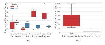
Fig. 11: Intersection congestion degree (ICD) and Region Congestion Degree (RCD) under congestion attacks after 60minutes simulation. The x-axis of (a) and (b) is the intersection denoted as A, B, C, D. The y-axis of (a) is the Intersection congestion degree (ICD), y-axis of (b) is the Region Congestion Degree (RCD). The attack vehicle is put on the Intersection C.
