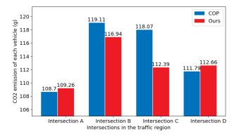
Fig. 8: The  $CO_2$  emission comparison of our method and the COP algorithm. The x-axis is the intersection denoted as A, B, C, D. The y-axis is the average of  $CO_2$  emission in 60-minutes simulation for each vehicle.
