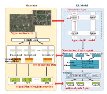
Fig. 4: Multi-agent reinforcement learning-based signal planning framework.
