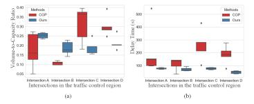
Fig. 10: Volume-to-Capacity Ratio (V/C) and Delay Time (DT) under congestion attacks after 60-minutes simulation. The x-axis of (a) and (b) is the intersection denoted as A, B, C, D. The y-axis of (a) is the Volume-to-Capacity Ratio (V/C), y-axis of (b) is the Delay Time (DT)(seconds). The attack vehicle is put on the Intersection C.
