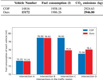
Fig. 7: The fuel consumption comparison of our method and the COP algorithm. The x-axis is the intersection denoted as A, B, C, D. The y-axis is the average of fuel consumption in 60-minutes simulation for each vehicle.
