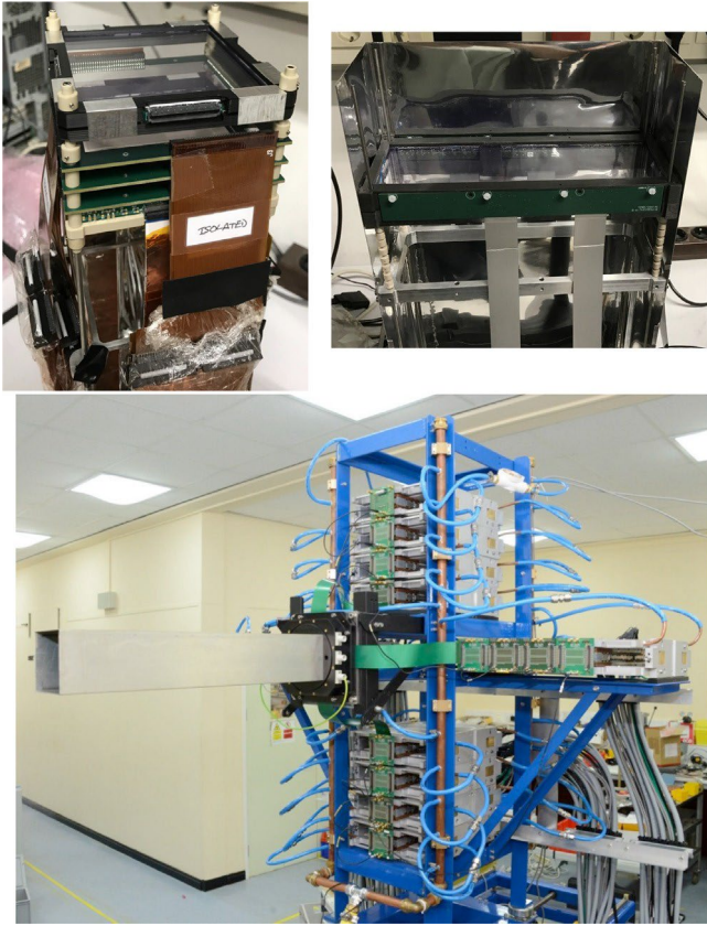
Fig. 3. Top photograph left: The arrangement of three layers of AIDA DSSD chips in the narrow configuration coupled to one of the \beta Plastic detectors (on top), ready to be inserted into the snout. Top photograph right: AIDA in the wide configuration. Bottom photograph: The built AIDA detector system: the snout on the left contains the several layers of the narrow 8 \times 8 \text{ cm}^2 DSSDs, while the blue frame hosts the electronics. The blue pipes contain the cooling medium for the electronics.
