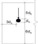
**Figure 2** a) Geometry and reinforcement of the strengthened beam with layers and dowels b) Minimum required cover for the dowels based on the Greek Code for Interventions
