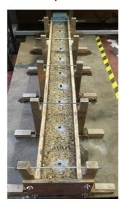
Figure 3 Beam with dowels ready for casting
