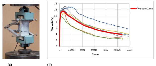
Figure 4 a) Dog bone specimen b) Experimental results from the direct tensile testing of UHPFRC
