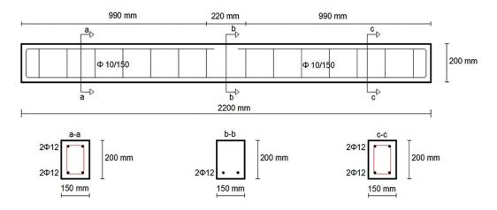
Figure 1 Geometry and reinforcement of the RC beams
